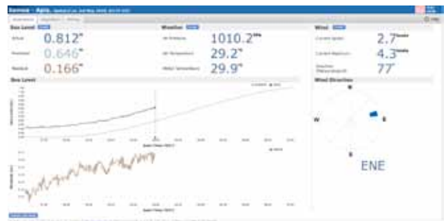
A dashboard view of real-time sea level and weather information from the Samoa tide gauge in Apia.
